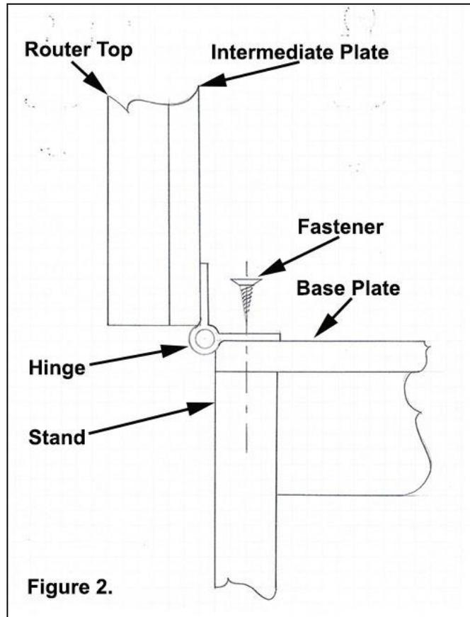
9. Secure base plate to stand. If wood stand, use 2 countersunk holes on hinge, together with 2 - #8 x 1 1/4" screws to secure base plate to stand and once position of base plate to stand is determined, drill and countersink 3 additional holes to accept 3 - #8 x 1 1/4" screws, two at base plate sides and one at forward section. (Minor adjustment may be required depending on thickness of stand cross rail).
