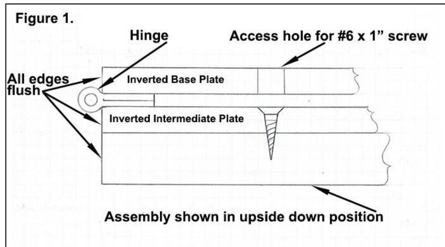
5. **NOTE:** If router table is phenolic, pilot holes are essential. Using access holes on base plate, drill pilot holes on underside of router table top. For #6 screws use 7/64" diameter drill. Use drill stop or tape as depth gauge to prevent full penetration of router table top, (do not drill pilot holes if router top is MDF).
